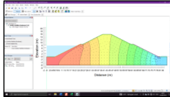
Gambar 18 Aliran Rembesan Water Total Head
