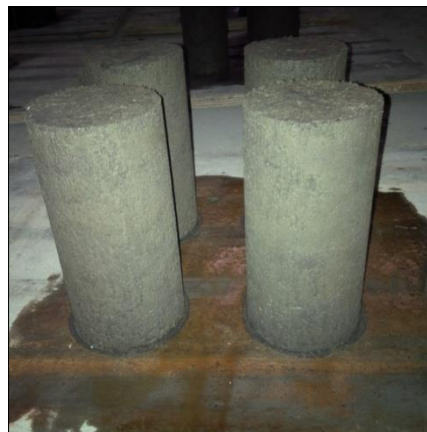
Figure 5. Concrete cylinder specimens (4 × 8 in)
