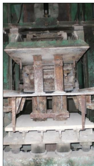
Figure 4. Production machine for dry-cast concrete
